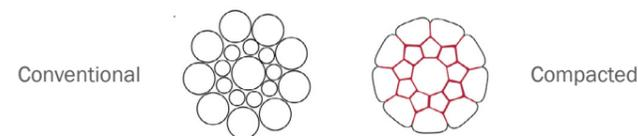
The compacted strand has very favourable internal contact conditions when compared with the point contact of round wires within a normal strand.
