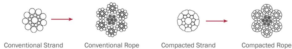
A Powerform<sup>®</sup> compacted rope is a steel wire rope which has been manufactured using individually compacted strands. During the compaction process the outside diameter of the strand is reduced and steel moves into the empty voids between the wires within the strand.
