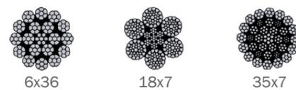
Usha Martin compacted ropes are referred to as "Powerform<sup>®</sup>" and are available in a number of constructions.
