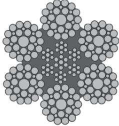
Warning : Hyflex 6x29Fi in Langs lay must only be used in applications where both ends are unable to rotate.
