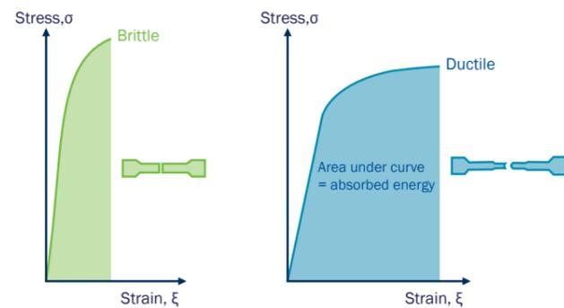
The graph compares the behaviour of wires at break with different strengths: the green line represents a brittle trend typical of high strength steel (over 2160 N/mm<sup>2</sup>). The blue line represents the typical trend of lower strength steel (1770 and 1960 N/mm<sup>2</sup>).
