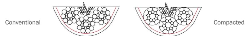
Exterior contact conditions are equally favourable. The smooth surface of the compacted rope offers a wider bearing surface to the sheave or drum groove.
